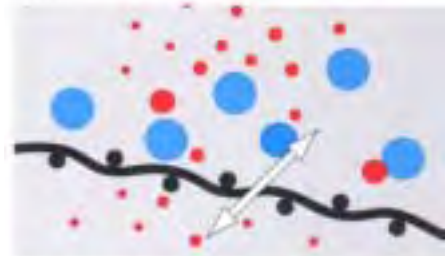
Material tends to become airborne on vibrating screening types because of the vigorous vertical motion.
