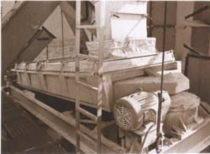
Model 552 ROTEX Grain Cleaner at The Pillsbury Co., Lilly Chapel, Ohio, cleaning corn and soybeans. This model has two independently fed surfaces, providing rates up to 15,000 BPH.
