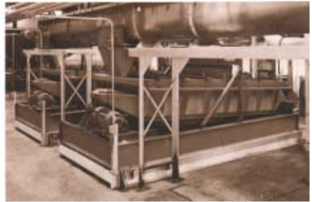
Model 722 ROTEX Grain Cleaners at Burge Corp., Cairo, Illinois, cleaning whole and cracked soybeans , at rates up to 9,000 BPH.
