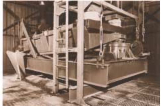
Model 722 ROTEX Grain Cleaner, incorporating air separation, cleaning 10,000 BPH of corn and wheat at W G. Thompson's Blenheim, Ontario Elevator.
